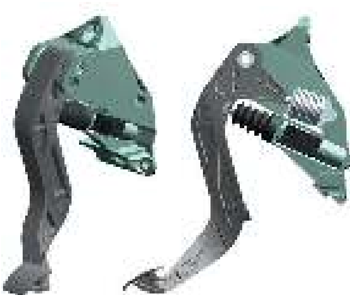
Figure 20 Pedal box for clutch operation made of plastic with integrated master cylinder and sensor
