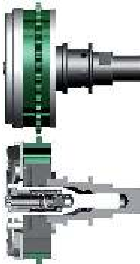
Figure 5 A positive example: The camshaft phasing unit is narrow, the sprocket is located on the camshaft
