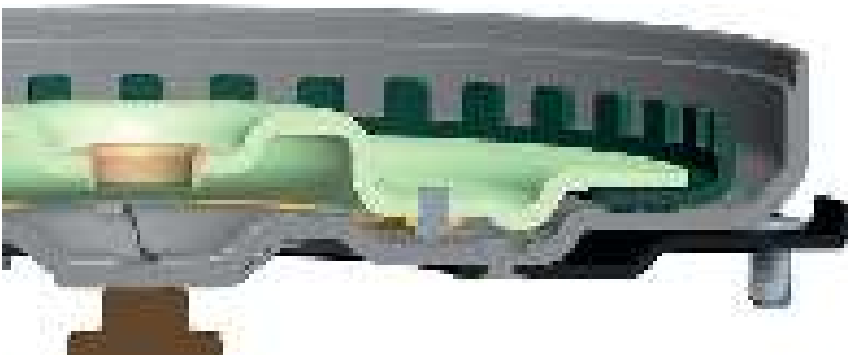
Figure 7 Schaeffler riveting at piston connection
